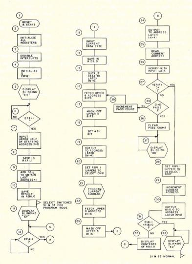
Fig. 7. Program sequence flow diagram.
